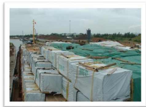
Example of staggered packs to help with safe discharge
