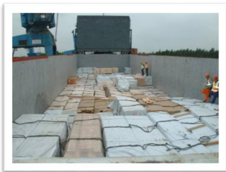
Discharging one layer at a time to reduce fall from height risk
