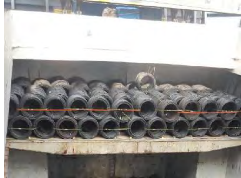
The WRIC tiers in the tween deck are lashed with steel bands. Steel bands are not elastic and cannot be secured to the vessels' bulkheads. Wire lashings shall be used instead.
