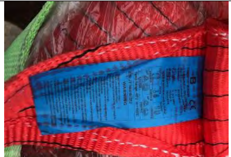
The slings for pre-slinging shall be certified and properly marked.
