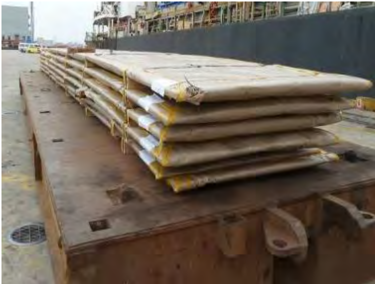
Packaged steel plate with protective wrapping and timber supports attached with steel strapping.
