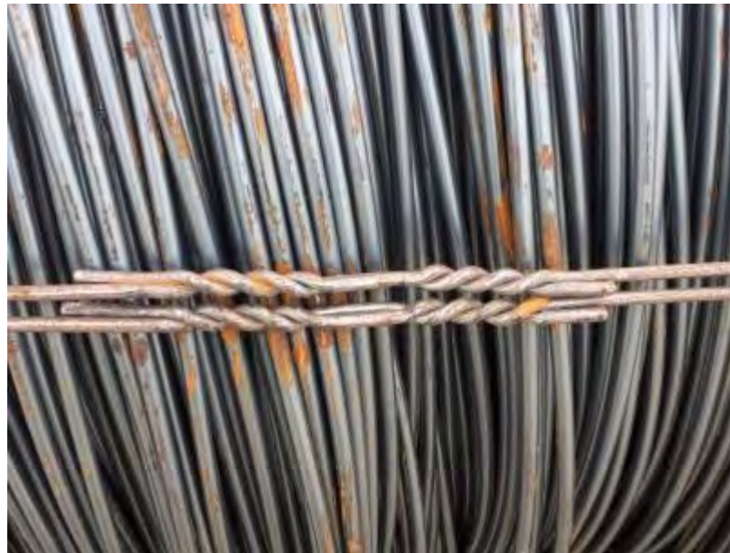
Bundling of WRICs with the use of double bundling wire rods and four twists.
