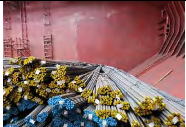
12m long rebar in the under-coaming space of a hopper-type bulk carrier. No dunnage. The stow is not levelled.
