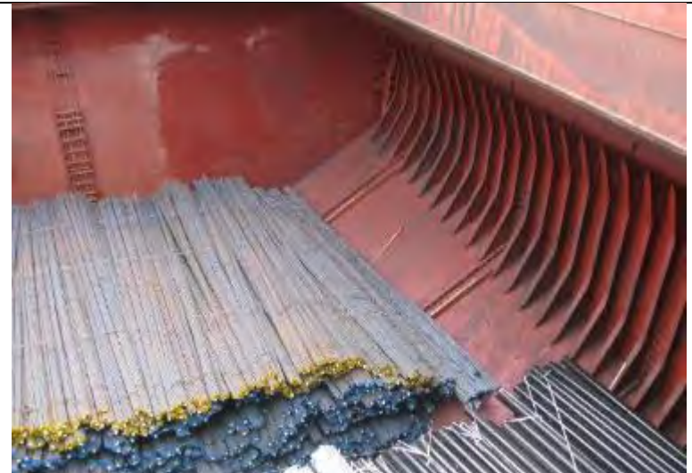
Shifted cargo at the discharging port. Under-coaming sloped stow of rebar. The hopper tank flares out to the middle of the hold.
