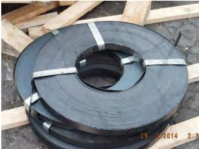
Metal strapping used for securing of pipes. The tightening shall be made with the use of pneumatic tools.
