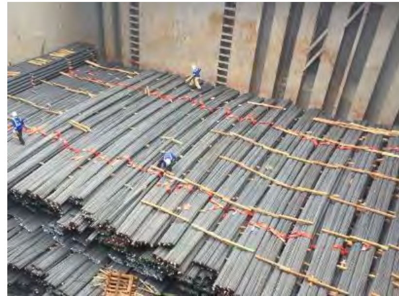
Loading. A stow of rebar bundles, pre-slung with nylon slings to assist the discharge operation. Dunnage is also used between the tiers.
