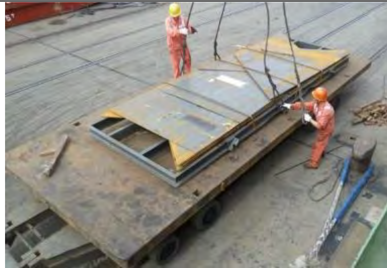
Bundled, palletised, pre-fabricated steel plates.
