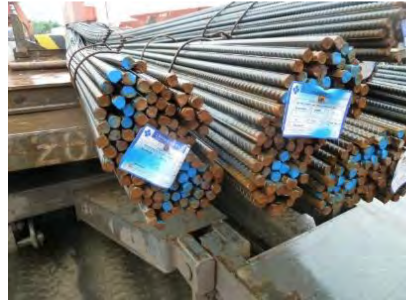
Bundling wires along the length of the bundles are not designed for lifting but can be used for tipping.
