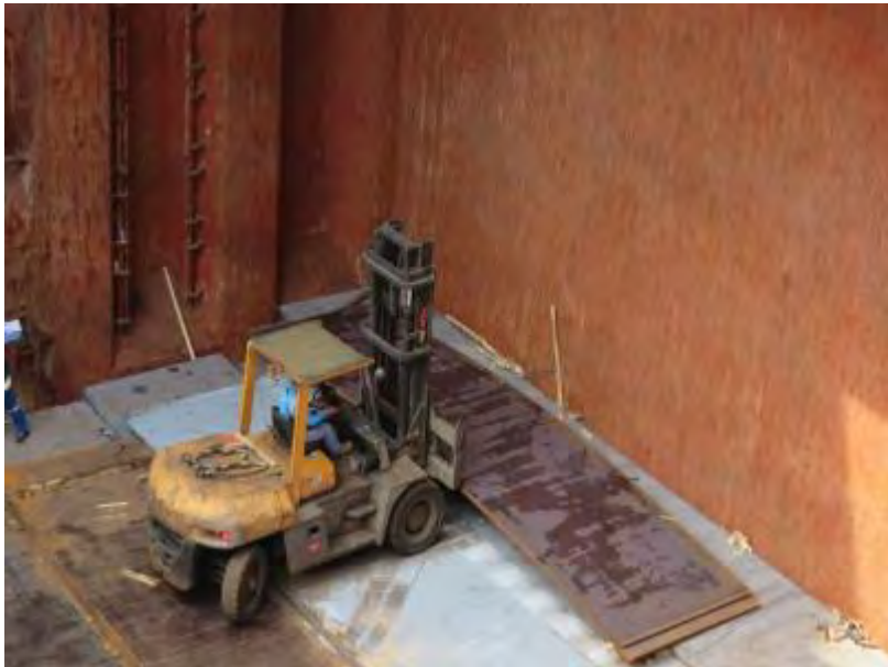
Steel plate being lifted, by a forklift truck, from the wing space of a bulk carrier.
