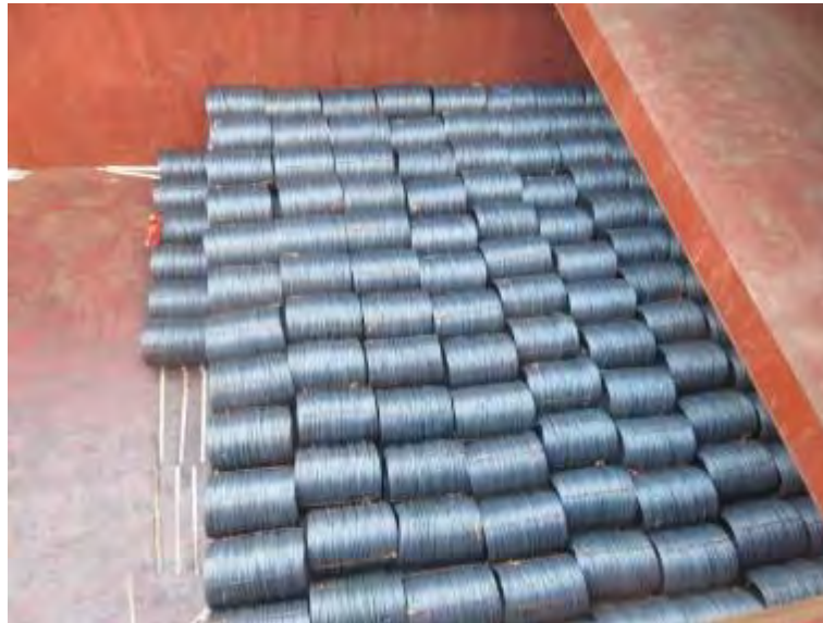
WRIC being stowed across the full width of a box-shaped cargo hold.
