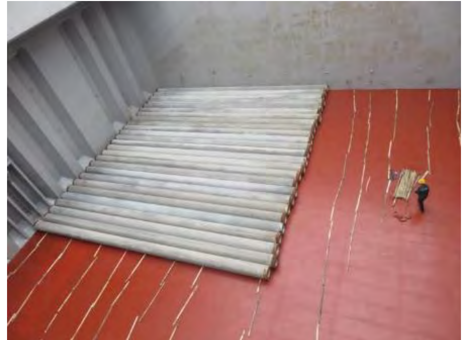
Dunnage being laid on the tank-top in preparation for the loading of loose pipe.
