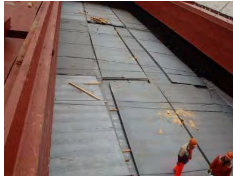
A level top stow of loose steel plates. Timber dunnage is used to secure the top plates, though this is not yet completed.
