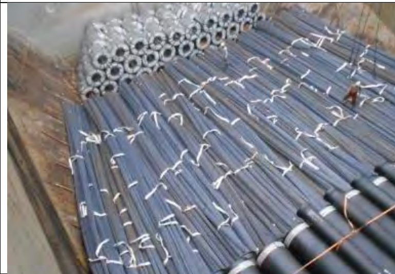
Pre-slung rebar is fanned out in way of the hopper tanks, but sufficient dunnage is placed on the hopper plating to prevent steel-on-steel contact.
