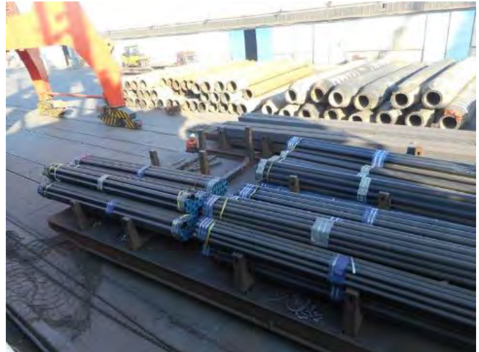
An assortment of pipes waiting to be loaded. Flanged, rubber-coated pipes in the background and bundles of finished steel pipes with pipe-end caps on the trailer.
