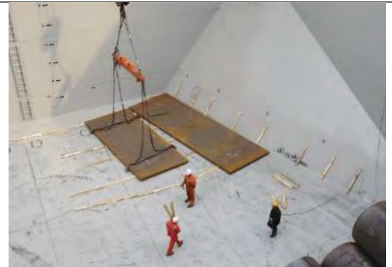
Dry bulk carrier with hopper-type cargo holds. Dunnage shall be used on the tank-top, side hopper tanks and bulkheads.
