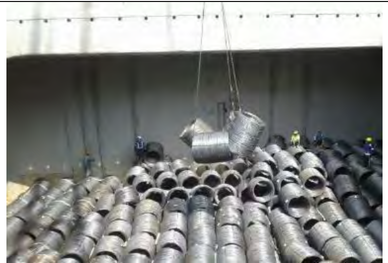
The coils will be off-loaded by the use of a single leg basket through WRICs. Four WRICs handled with two wire slings.
