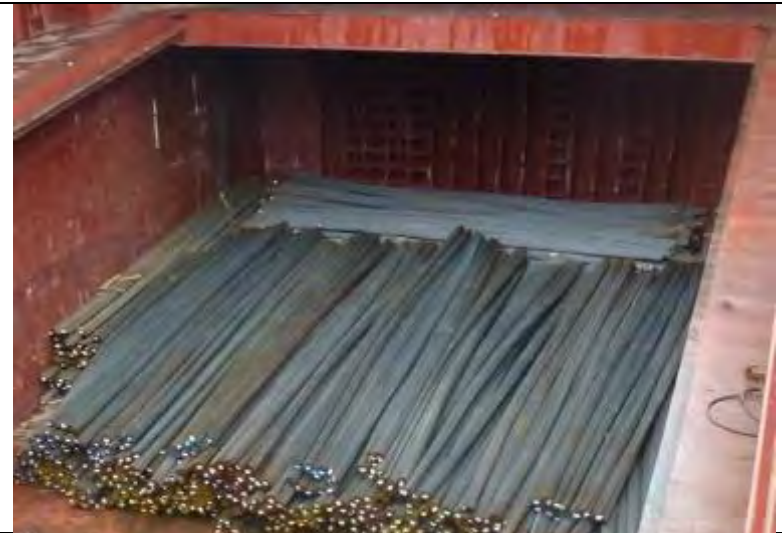
Rebar stowed athwartships in the under-coaming area requires a forklift truck for it to be discharged. No pre-slung and no dunnage between the tiers was used.
