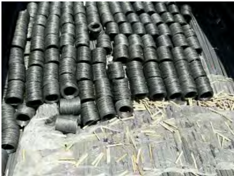
WRICs loaded on top of rebars segregated with plastic sheets.
