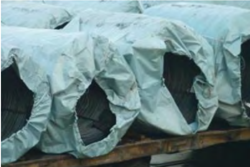
Partially protected WRIC secured with strapping bands. The outer canvas/plastic cover offers some protection from the elements.
