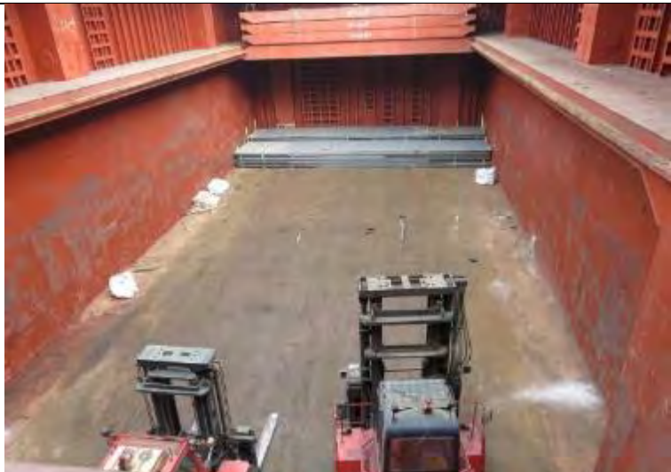
General cargo vessel with box-type cargo compartments. Lower hold and tween deck. Athwartships loading. Under-coaming loading.
