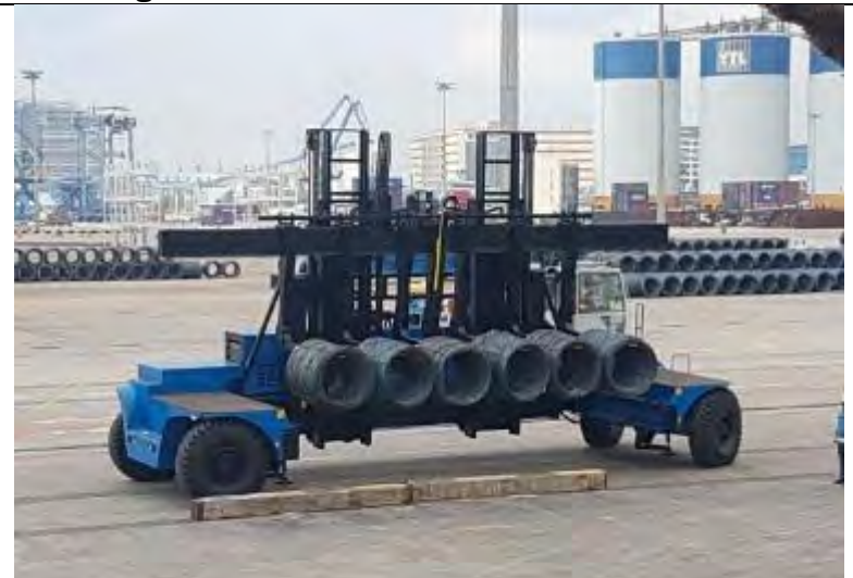
For example, Jurong Port has a multi-fork side-loader for transport from the quay to the storage area.
