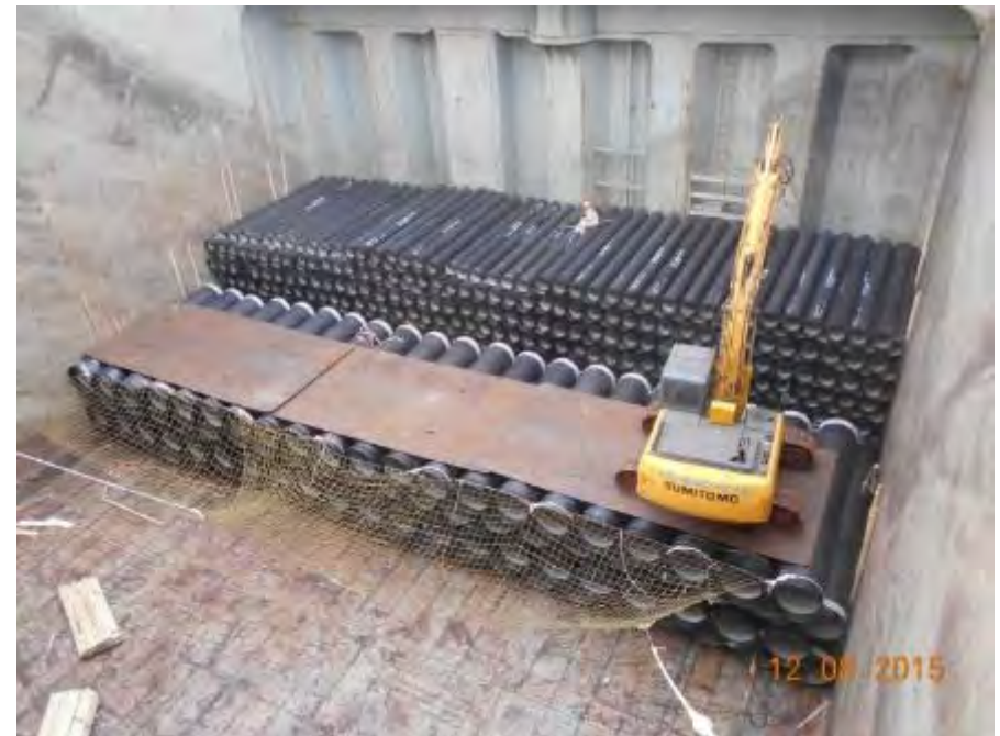
Two uniform stows of pipes. Note that the swaged ends are stowed at opposite ends on alternate layers; the faces are stepped accordingly.
