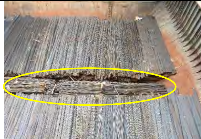
Bad mixed stow of 12m long rebar without dunnage and pre-slinging. There is no clearance between the fore and aft stows with athwartships cargo stowed in between.
