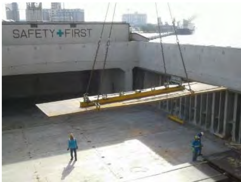
C-hooks and a spreader used for the off-loading of steel plates.
