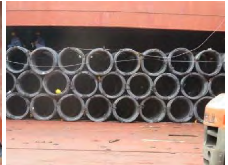
WRIC loaded in the 'tween deck space. The lashing gang are securing the top tier of the face of the stow.
