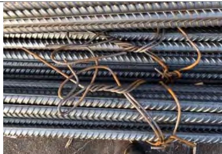
Lifting bundles by the bundling wires can lead to loosen bundles and/or broken straps, increasing the difficulty for discharge and the risk of damage.
