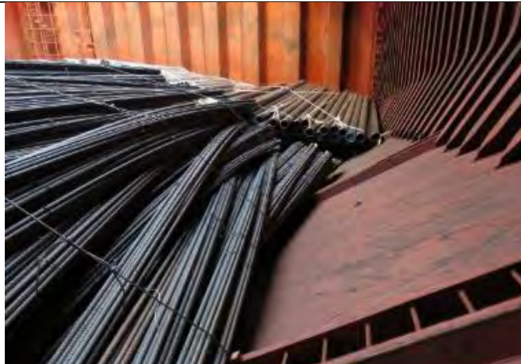
Shifted cargo at the discharging port. Bad pyramid stow of 12m long rebar without dunnage. Shifting of the rebar inside the under-coaming space.
