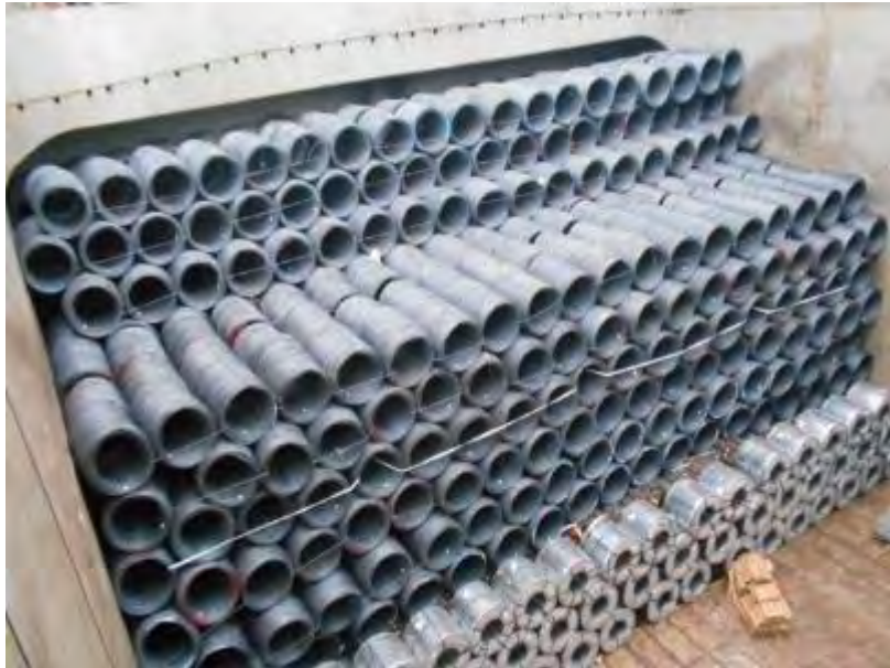
The tiers of the stow have been lashed back with wires to the after bulkhead. The height of this stow is significant.
