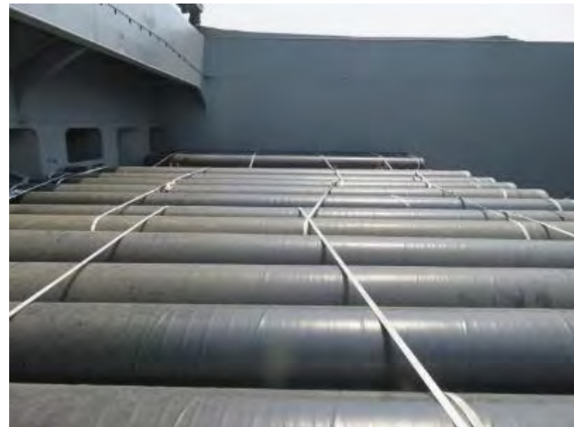
Nylon web strapping used to lash a stow of medium size pipes. The lashing is made only on the top tier of pipes in a box-shape cargo compartment.
