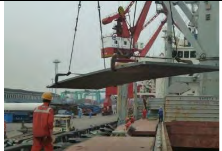
Loading of steel plates with 'C' clamps.
