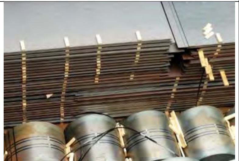
Good application of dunnage for steel plates. It is acceptable to use short hardwood dunnage pieces instead of long bars.
