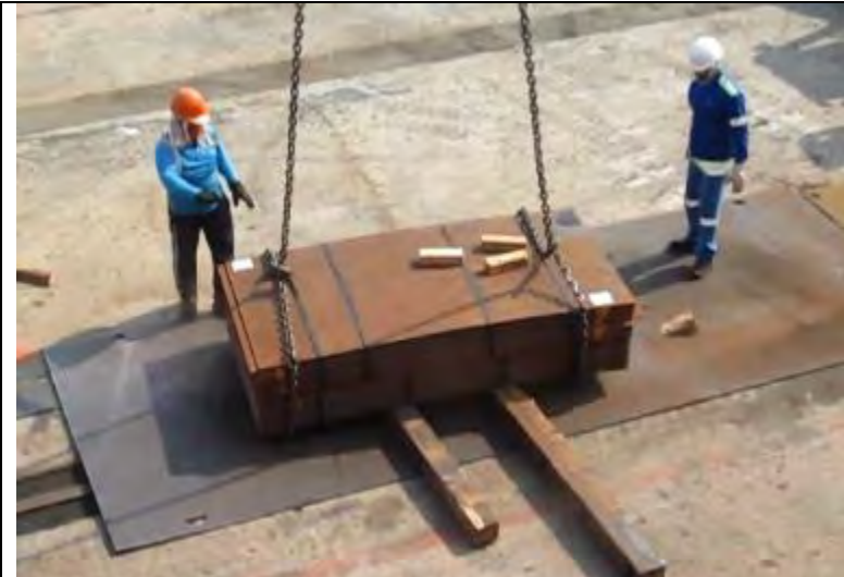
Bundled steel plates ready for loading. Choke hitch chain sling in use.
