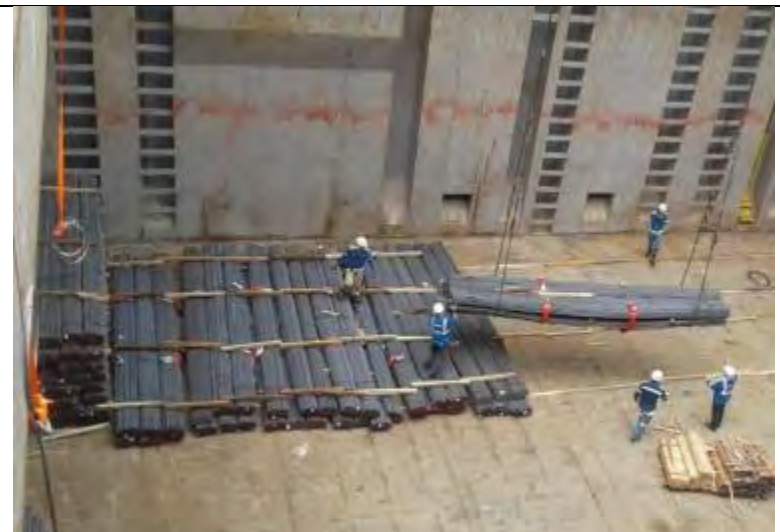
The tank-top is prepared with dunnage prior to loading. Dunnage and lashing wires have been pre-laid. The first cargo is loaded in the under-coaming areas.
