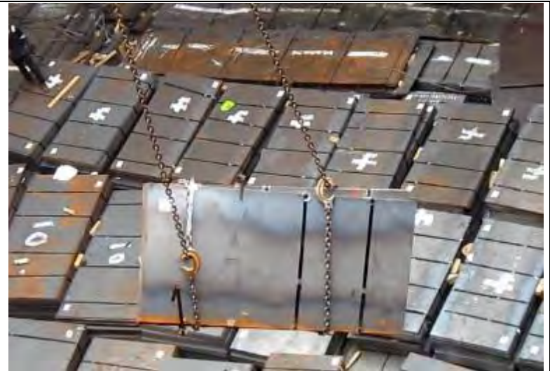
Bundled steel plates. Broken steel straps. Incorrect choke hitch application.
