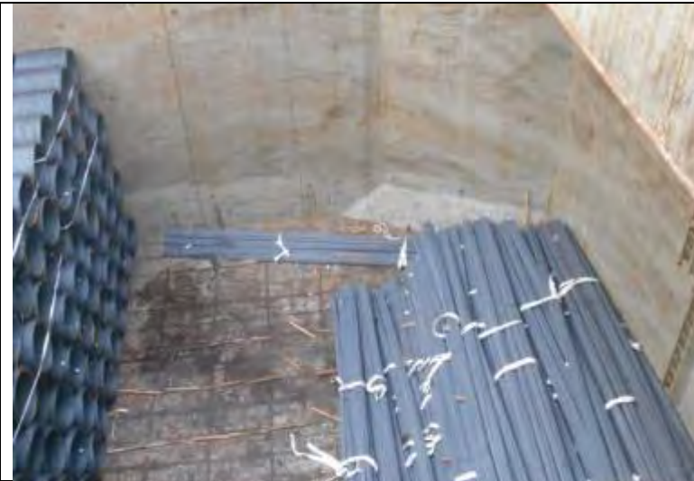
Pre-slung rebar is often stowed athwartships due to the constraints of the space available for loading
