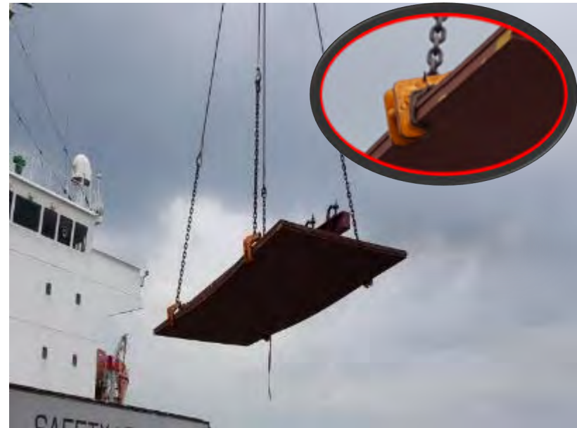
'C' hooks used for off-loading.
